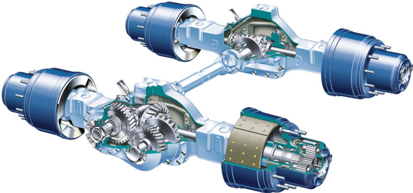
**RT3312 is a tandem axle with hub reduction, dimensioned for an engine torque of 3550 Nm. The maximum axle loading is 33 tons and the combination weight is 120 tons.**
