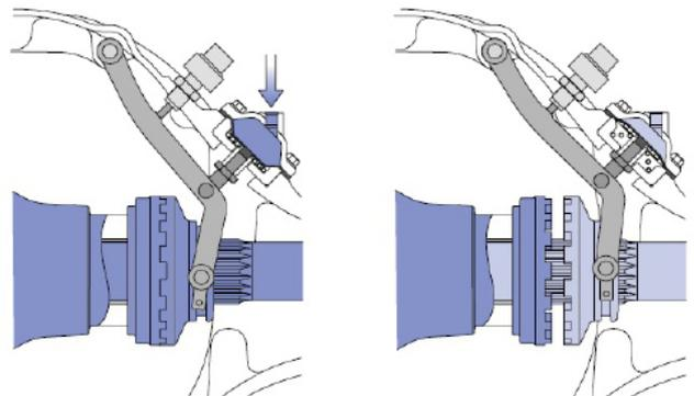
Differential lock engaged (rear axle)
